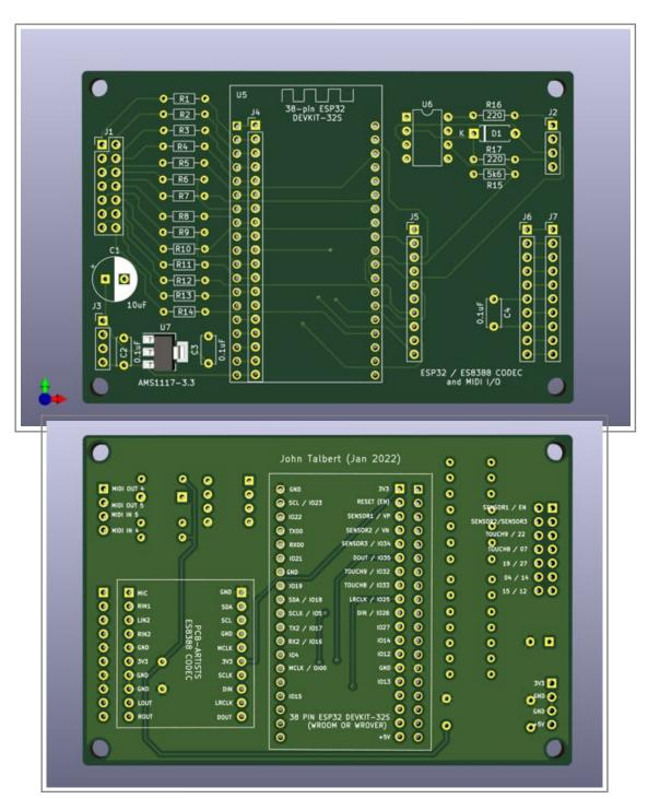
The central device on the PCB is the ESP32-DEVKITC-32D. This is a 39 pin module with a USB connection used to both program and power the ESP32 microprocessor. There are several versions of this board. The PCB board has an extra 19 pin header to accommodate two different sizes of the DEVKIT with pin widths of 22mm or 25mm.
