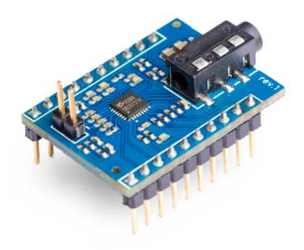
One side has all the digital connections to the ESP32 including the I2C Bus, the I2S Bus, and the System Clock. The other side has all the analog Audio connections, duplicated on a second 10-pin header. These include 2 audio outputs, 4 audio inputs, Circuit Ground, and 3.3volts. Two additional outputs are connected to a stereo headphone jack mounted on the Codec board.
