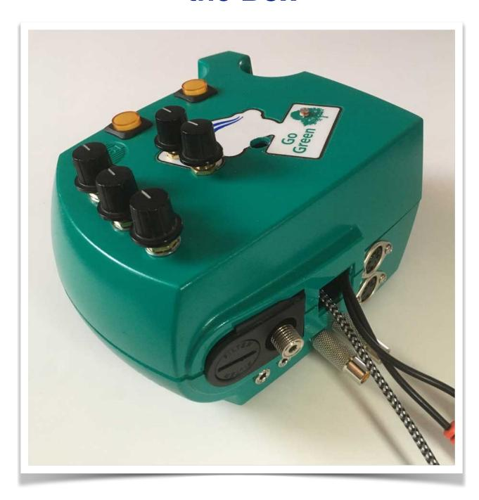
The PCB Codec board was mounted in the box shown above along with a number of controller devices and audio jacks connected by ribbon cable from the various board edge connectors.
